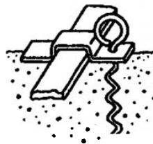
Figure 3.1: Auger Style Anchor
